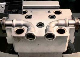
TUBEFORM: high-productive tube-endforming machine producing 2 tubes at a time.
